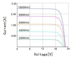
SUNWORTH solar modules have superior performance under low solar irradiation condition ( 200W/  $\rm m^2$  (AM1.5, 25  $^{\circ}C)$
